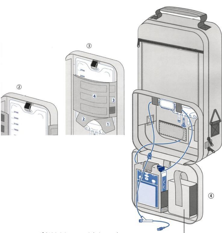
If CADD-Prizm pump is being used, \_\_ the power pack will fit into this pocket
